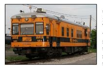
A form of X-ray is even used by railroads to find internal defects in tracks. Thanks to Elmer Sperry who invented this technology nearly a century ago, train travel is safer and more reliable. A Sperry rail detector vehicle can inspect
